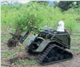
Electro-mechanical extraction of the coca plant
