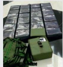
Portable photovoltaic source
