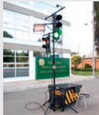
Portable device for vehicle flow signalling
